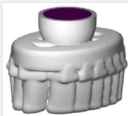
Ceramic mold automatically created in the PolygonSoft preprocessor (SKBT LLC)
